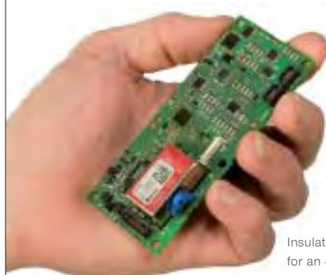
Insulation monitoring device for an e-vehicle
