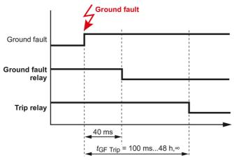
Figure 7-1: Ground fault relay timing diagram
