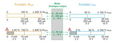
Figure 4-5: Assignment of measured value to output signal
