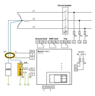
Figure 4-1: Star configuration (up to 690 V)
