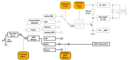
Figure 6-2: Configuration Digital 1 as NGR method
