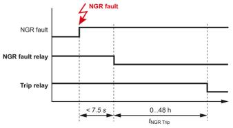
Figure 7-2: NGR fault relay timing diagram
