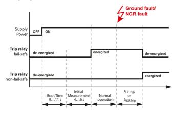
Figure 7-3: Timing diagram device start
