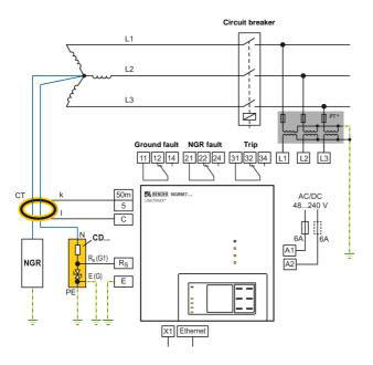
Figure 4-2: Star configuration (Usys > 690 V)
