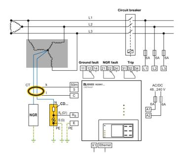
Figure 4-4: Artificial neutral with a zigzag transformer
