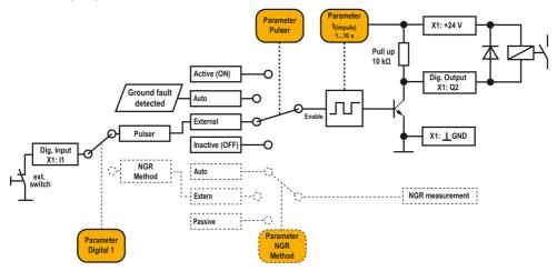
Figure 6-1: Configuration Digital 1 as pulser
