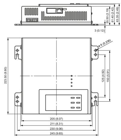
Figure 3-2: Dimension diagram and mounting position NGRM7...; mm(in)
